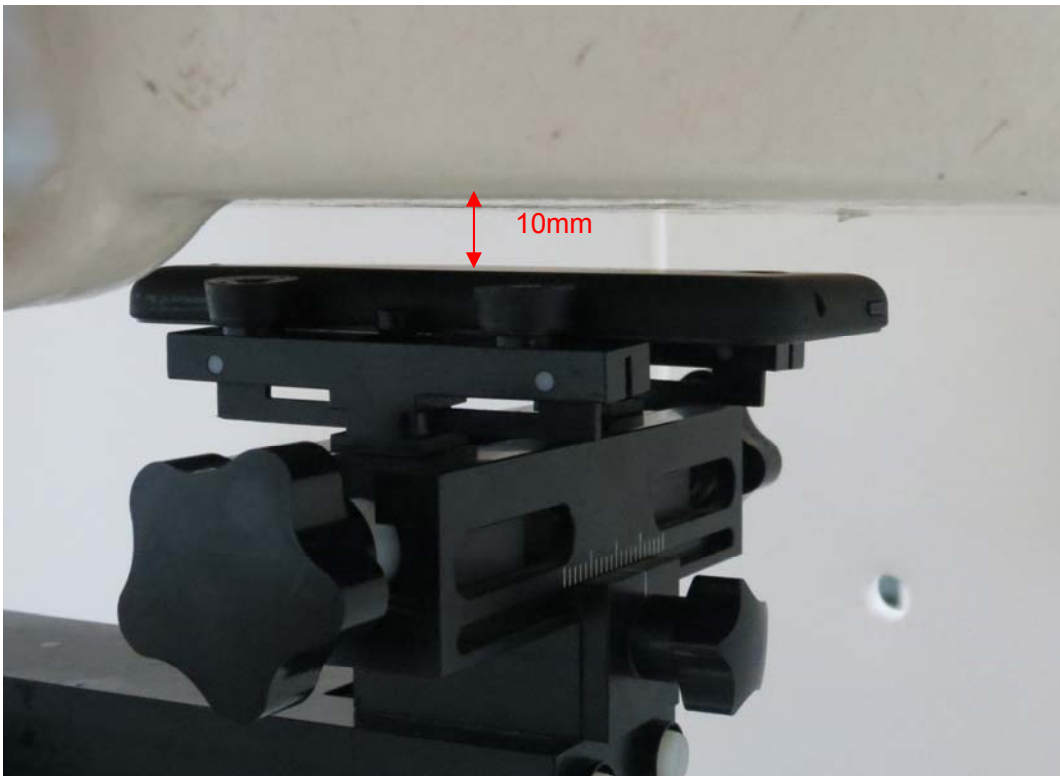
Picture 17: Back Side, the distance from handset to the bottom of the Phantom is 10mm
