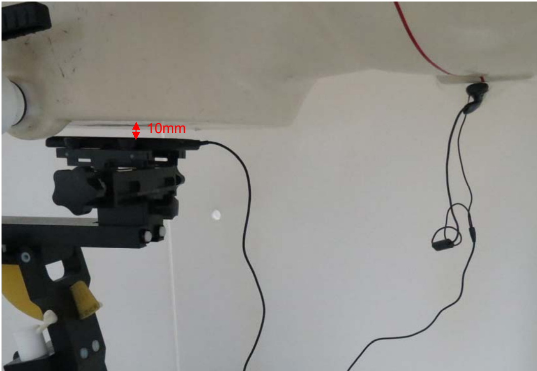
Picture 23: Back Side with Earphone, the distance from handset to the bottom of the Phantom is 10mm
