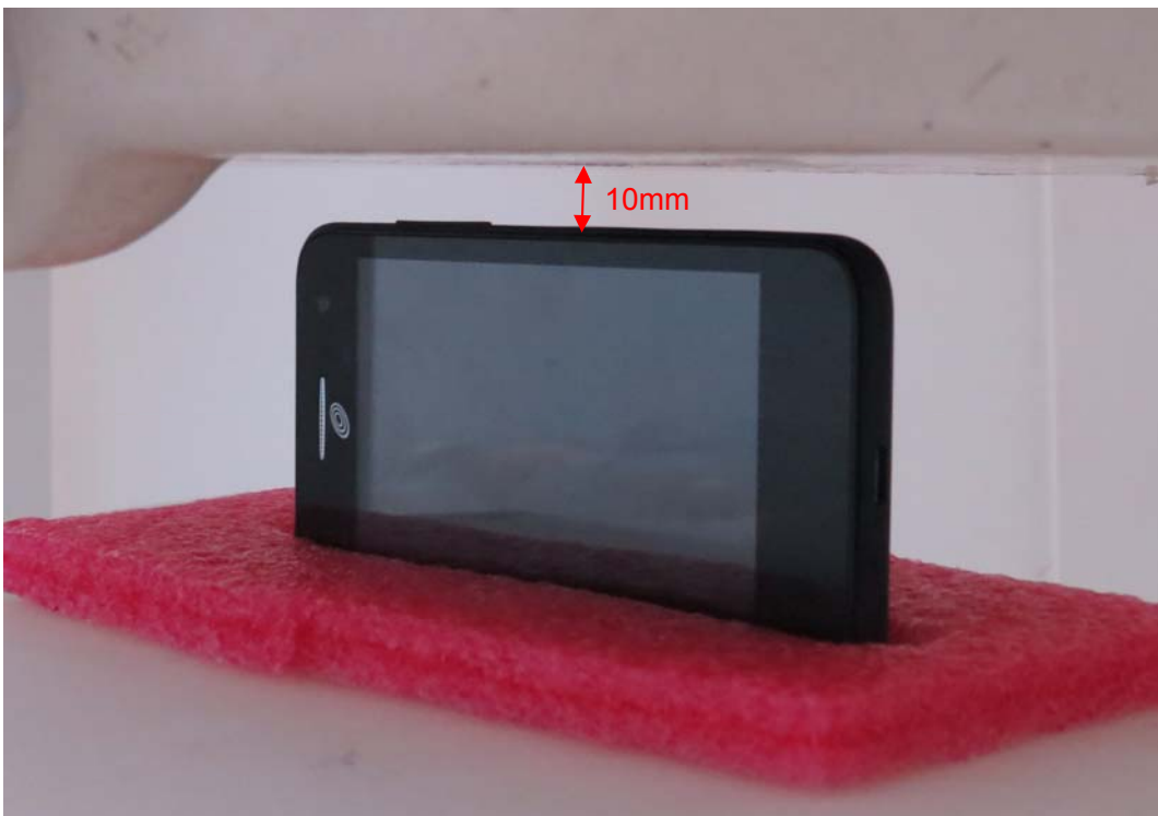
Picture 20: Right Edge, the distance from handset to the bottom of the Phantom is 10mm
