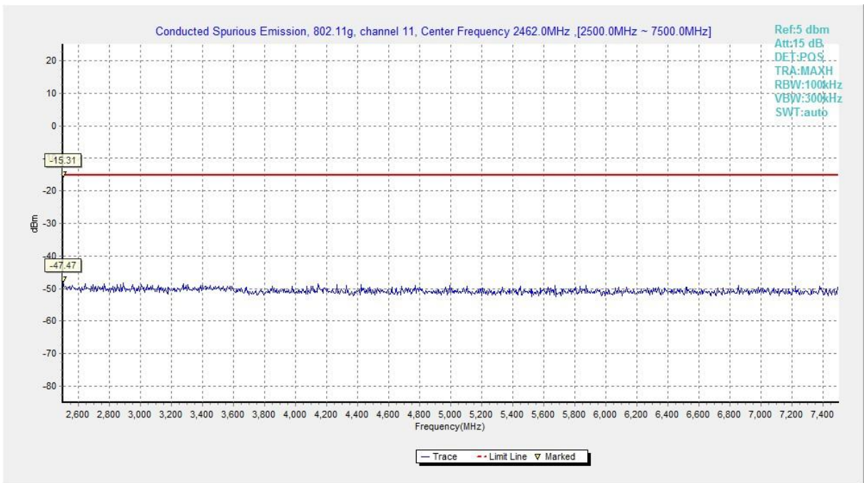
Fig.A.6.1.44 Conducted Spurious Emission (802.11g, Ch11, 2.5 GHz-7.5 GHz)
