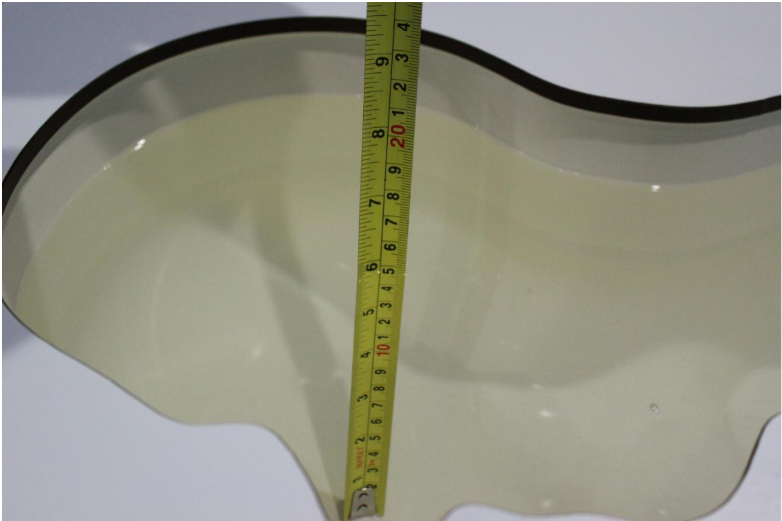
Picture 7-9 Liquid depth in the Head Phantom (5GHz)
