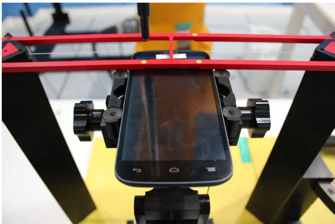
Picture 2: EUT Positioning for RF
