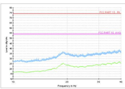
Figure A.5 Radiated Emission from 1GHz to 4GHz
