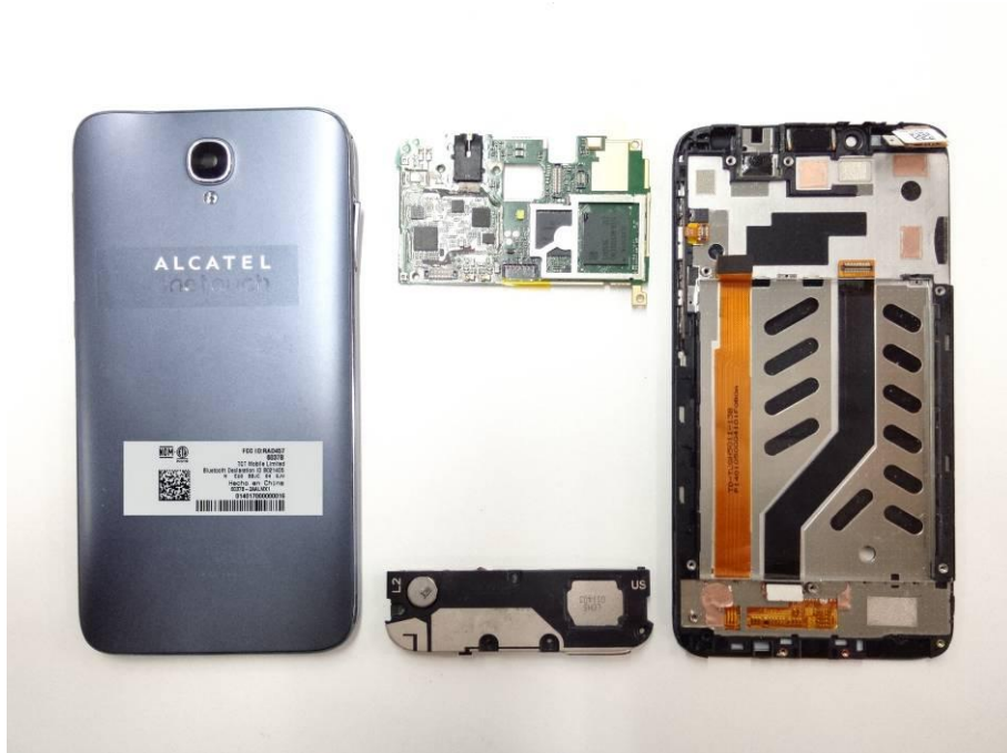
Pic A-3 Mobile phone Disassembly
