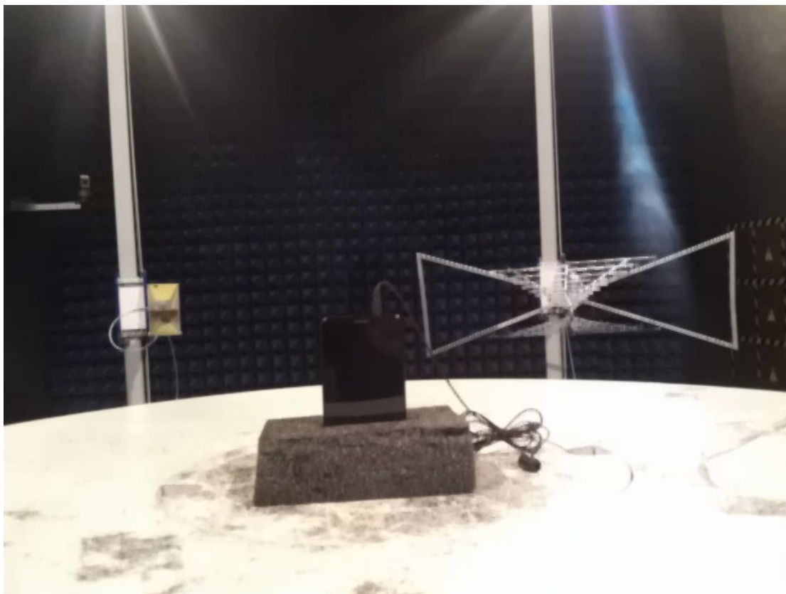
Radiated Spurious Emissions Test setup
