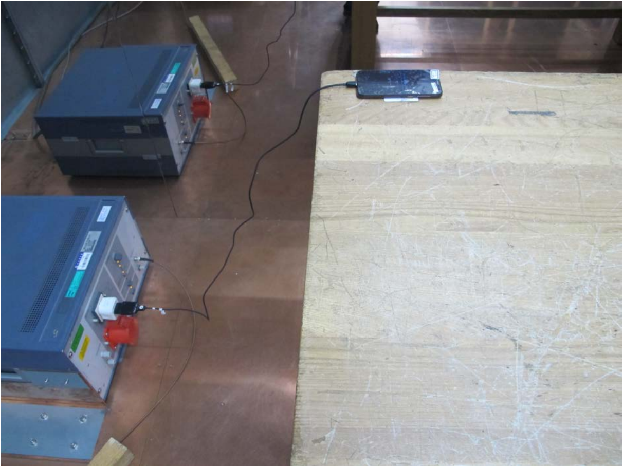
Picture C-3: Conducted Emissions Measurements
