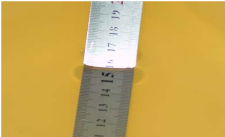
Liquid depth for SAR Measurement
