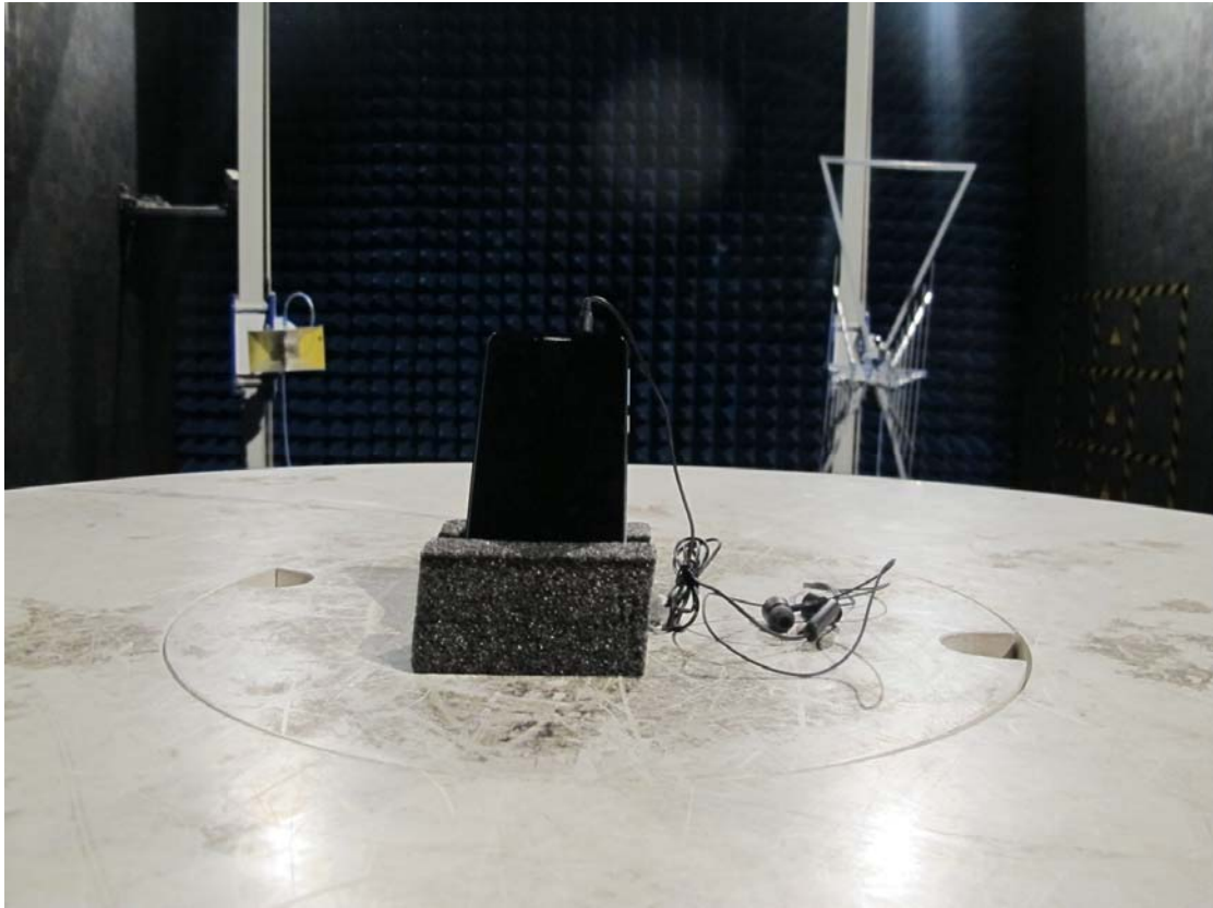
Radiated Spurious Emissions Test setup
