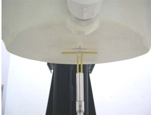
Fig 7.2 Photo of Dipole Setup
