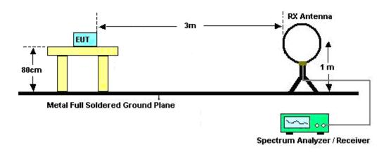
For radiated emissions from 30MHz to 1GHz
