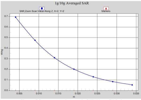
Fig. 7-1 Z-Scan at power reference point (WCDMA1900 CH9538)
