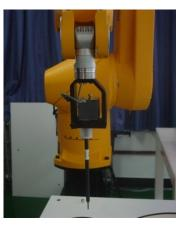
**Picture C.3 E-field Probe**
