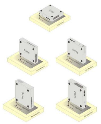
Picture D.5 Test positions for desktop devices
