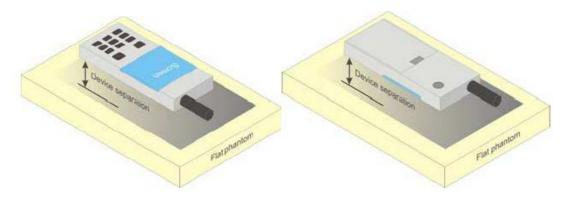
Picture D.4 Test positions for body-worn devices
