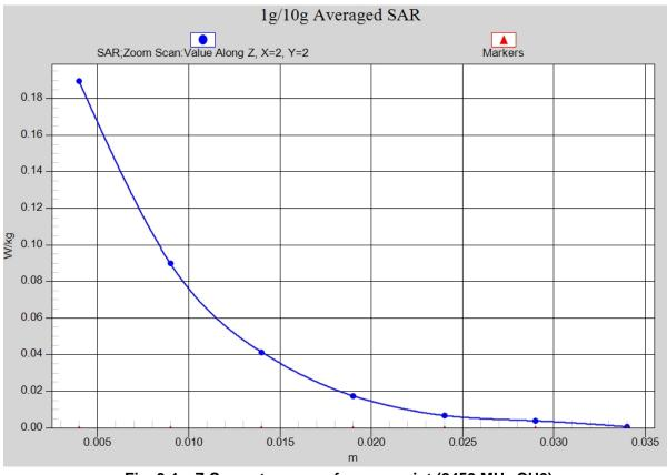
Fig. 9-1 Z-Scan at power reference point (2450 MHz CH6)
