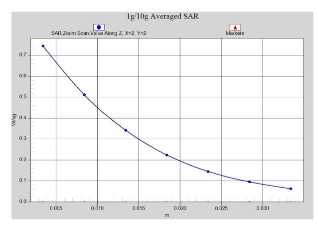
Fig.4-1 Z-Scan at power reference point (1900 MHz CH512)
