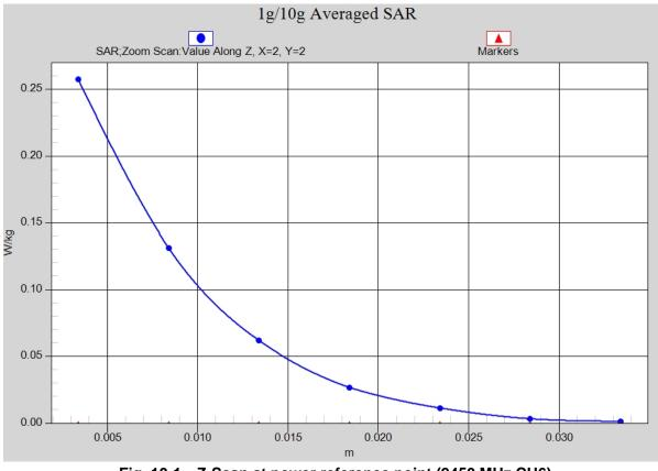
Fig. 10-1 Z-Scan at power reference point (2450 MHz CH6)
