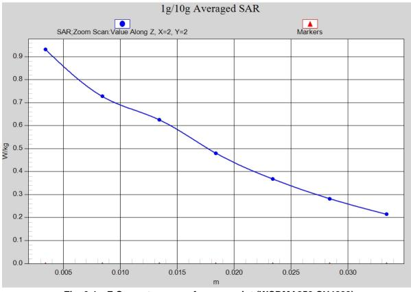
Fig. 6-1 Z-Scan at power reference point (WCDMA850 CH4233)
