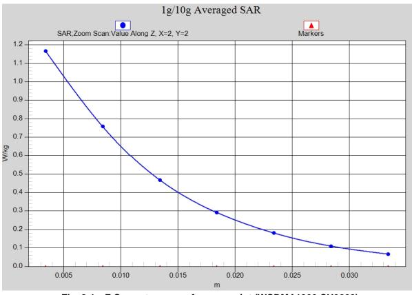
Fig. 8-1 Z-Scan at power reference point (WCDMA1900 CH9262)
