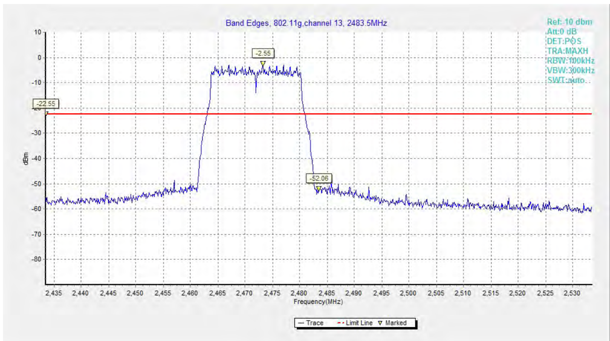
Fig.A.5.8 Band Edges (802.11g, Ch 13)
