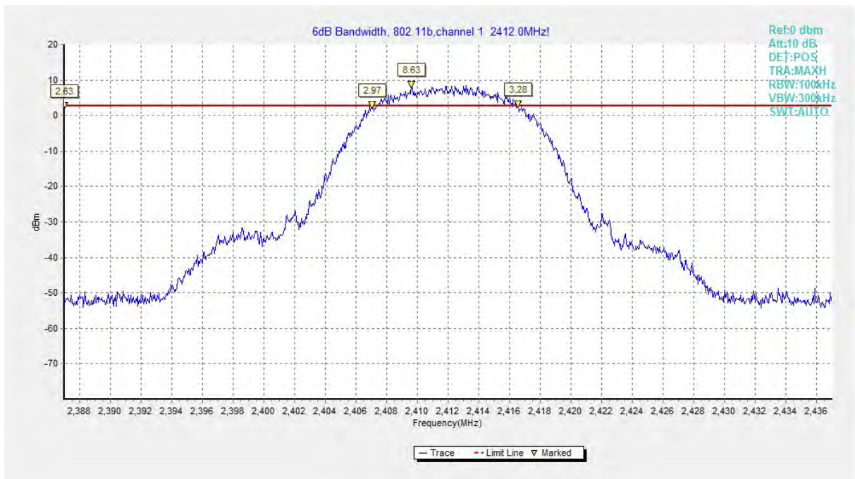
Fig.A.4.1 Occupied 6dB Bandwidth (802.11b, Ch 1)
