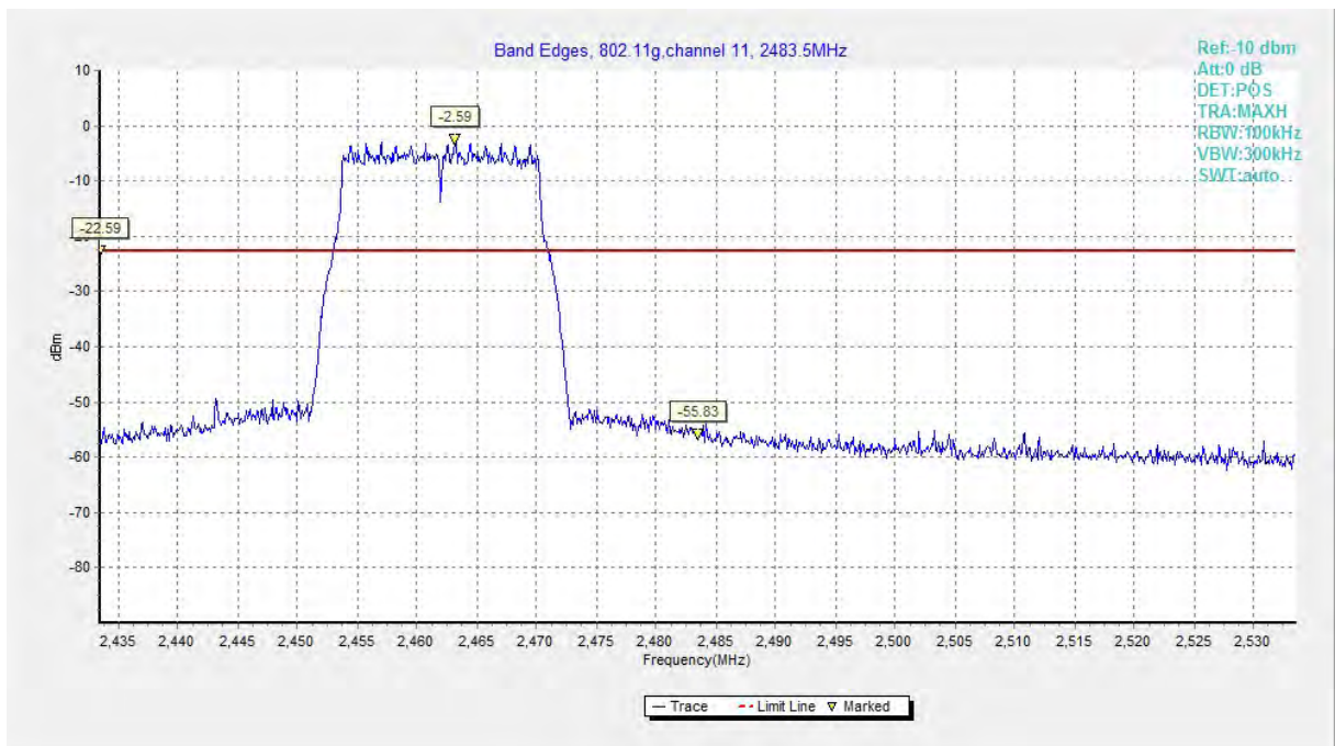
Fig.A.5.6 Band Edges (802.11g, Ch 11)
