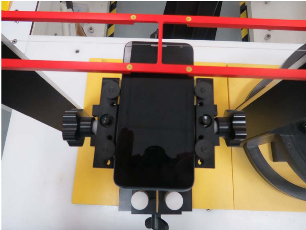
6036A HAC test setup photo RF Emission
