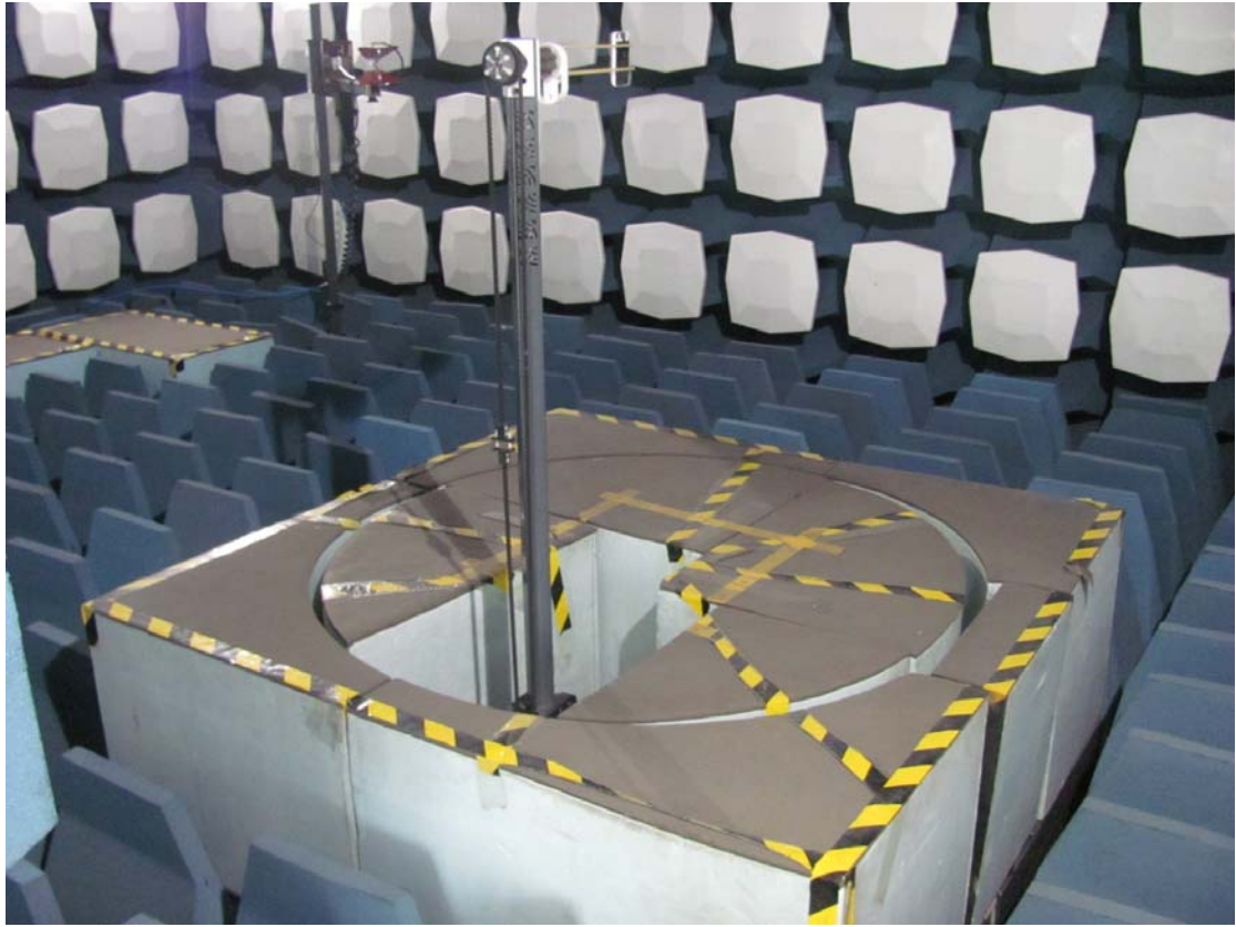
Pic F-2 Radiated Spurious Emission Test Layout
