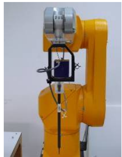
Figure 3. EX3DV4 E-field probe
