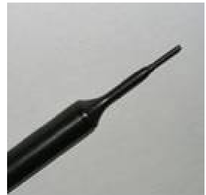
Figure 2. EX3DV4 E-field Probe
