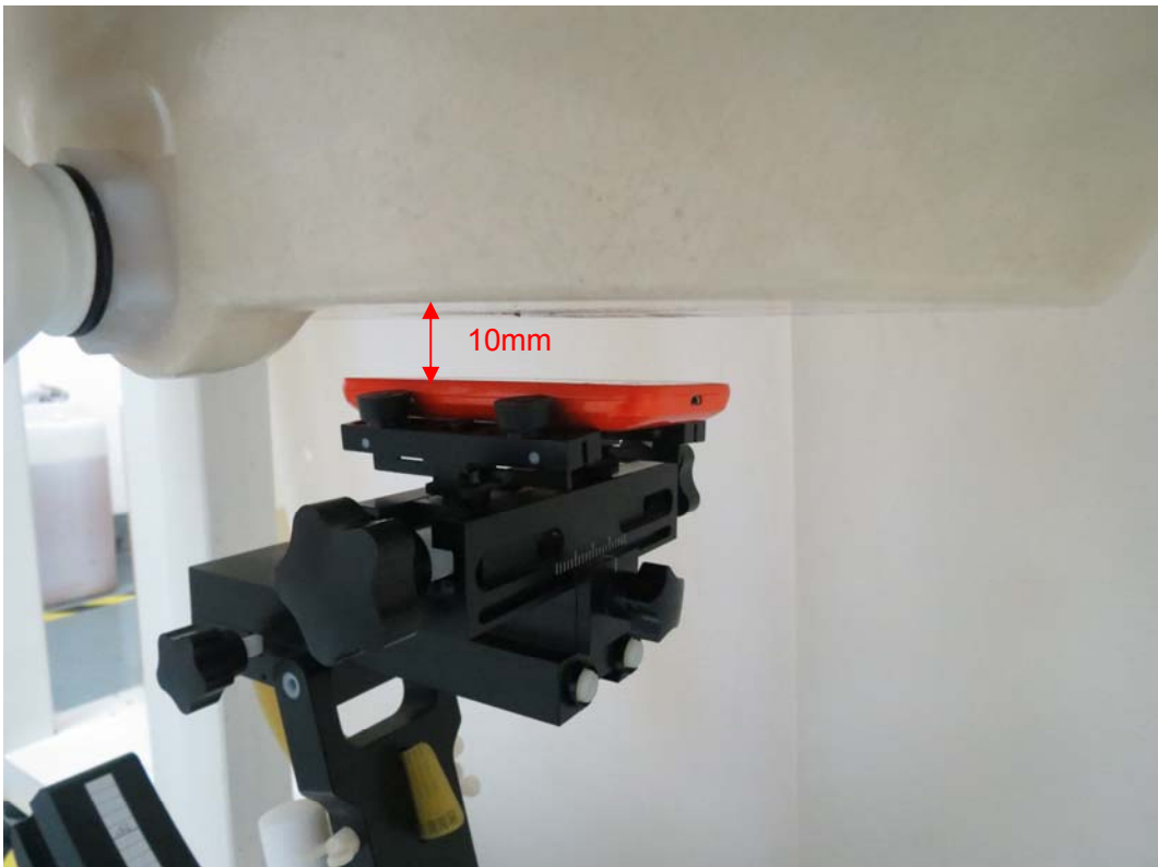
Picture 14: Front Side, the distance from handset to the bottom of the Phantom is 10mm
