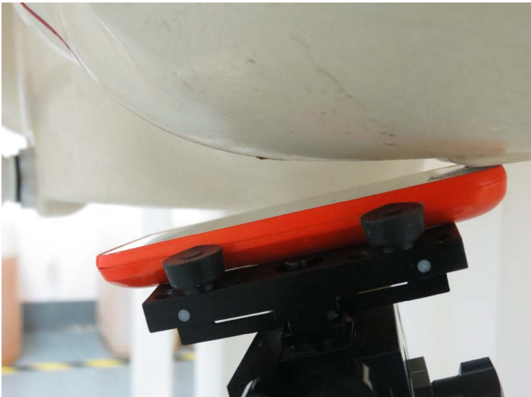
Picture 10: Left Hand Tilt 15 Degree Position
