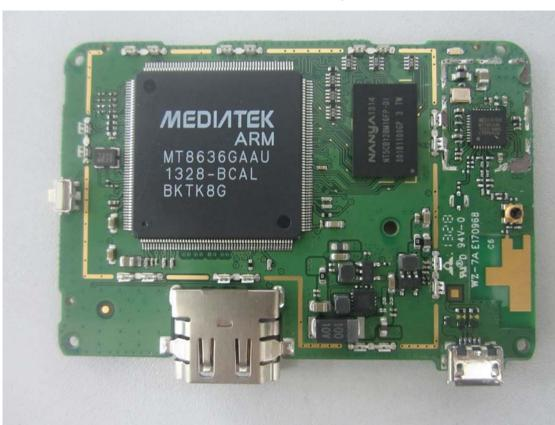
4. Mainboard front view without shielding
