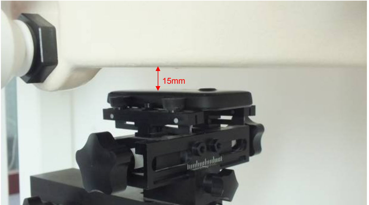
Picture 9: Back Side, the distance from handset to the bottom of the Phantom is 15mm
