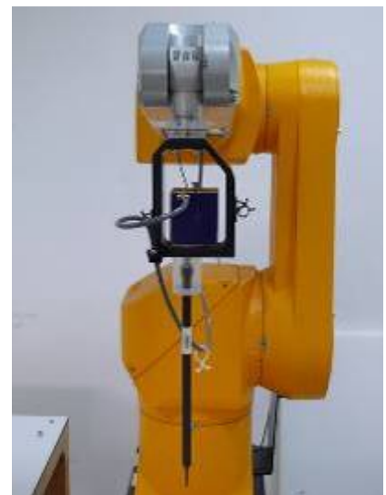
Figure 3. EX3DV4 E-field probe
