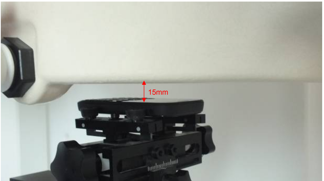
Picture 10: Front Side, the distance from handset to the bottom of the Phantom is 15mm
