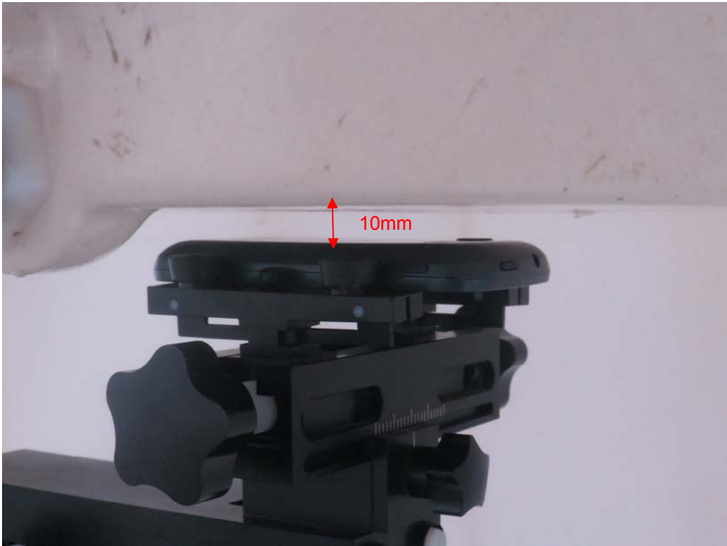
Picture 13: Back Side, the distance from handset to the bottom of the Phantom is 10mm
