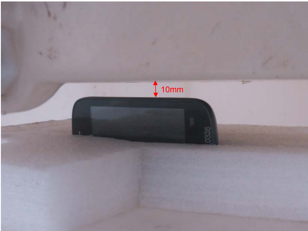
Picture 16: Right Edge, the distance from handset to the bottom of the Phantom is 10mm
