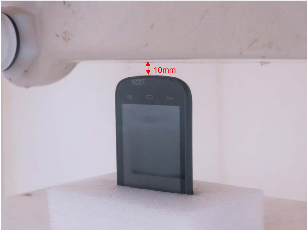
Picture 18: Bottom Edge, the distance from handset to the bottom of the Phantom is 10mm
