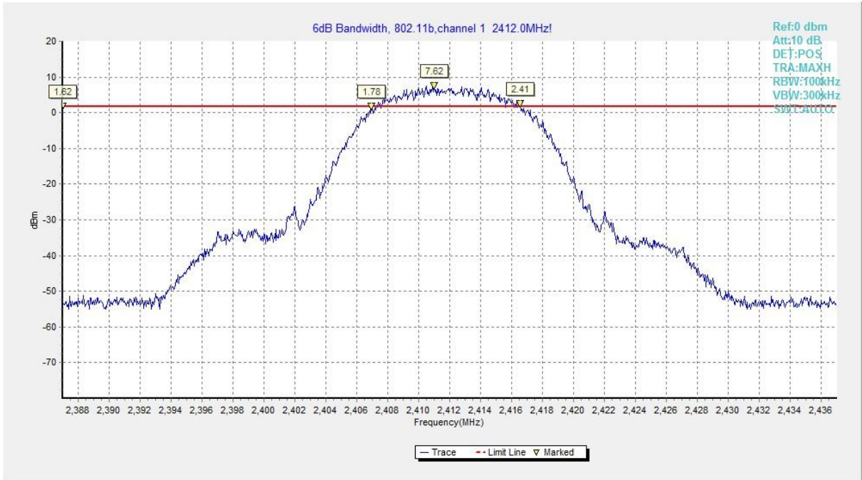
Fig.A.4.1 Occupied 6dB Bandwidth (802.11b, Ch 1)
