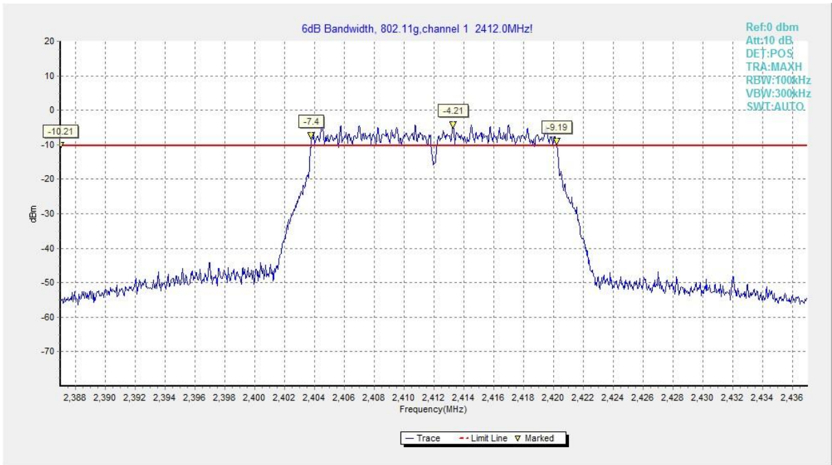
Fig.A.4.4 Occupied 6dB Bandwidth (802.11g, Ch 1)
