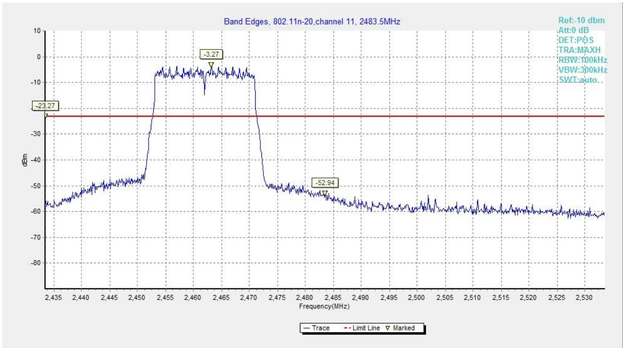
Fig.A.5.6 Band Edges (802.11n-HT20, Ch 11)
