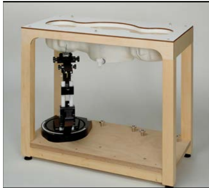
Picture C.10: SAM Twin Phantom
