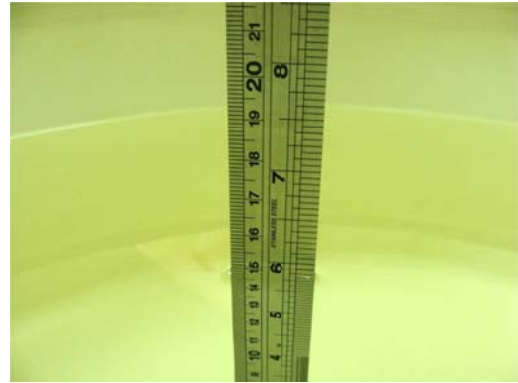
Fig 6.2 Photo of Liquid Height for Body SAR
