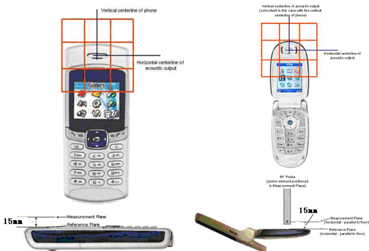
Figure 5 WD reference and plane for RF emission measurements
