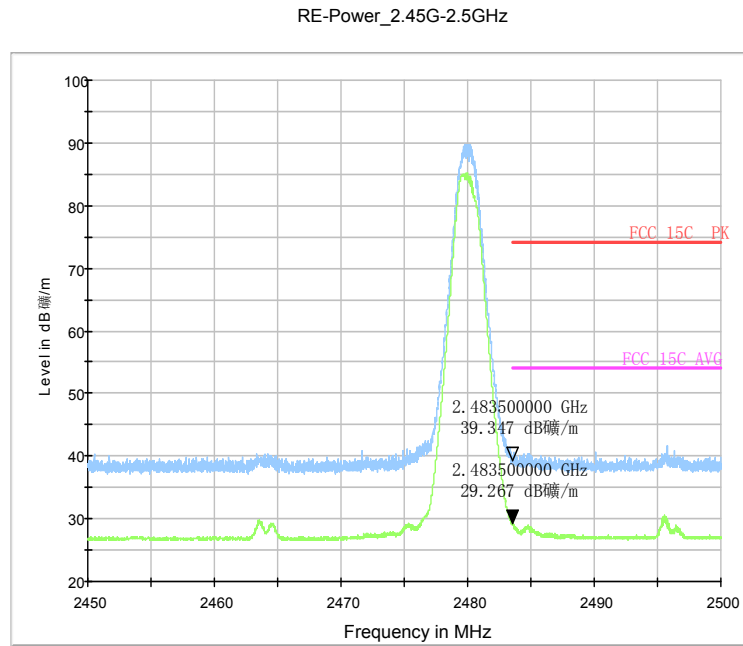
Fig.83. Radiated emission (Power): 8DPSK, high channel
