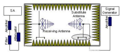
In the chamber, an substitution antenna for the frequency band of interest is placed at the reference point of the chamber. An RF Signal source for the frequency band of interest is connected to the substitution antenna with a cable that has been constructed to not interfere
