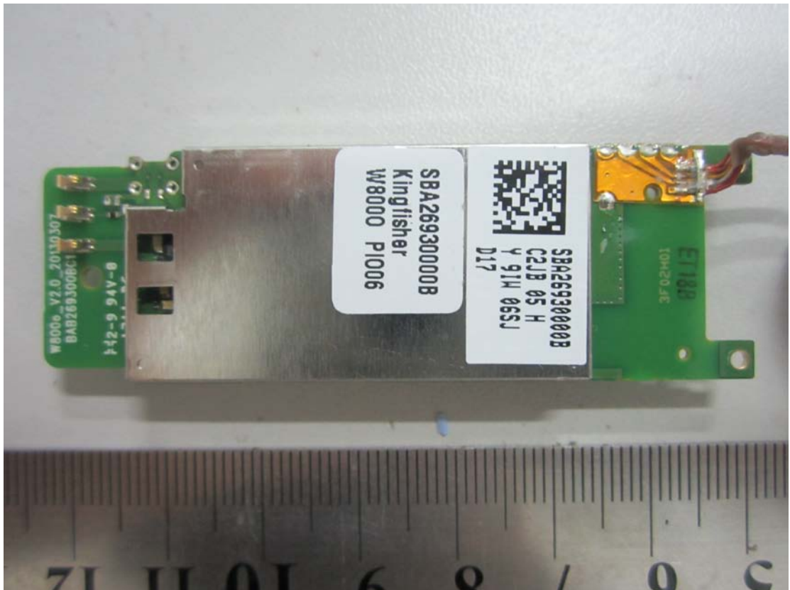
3. Mainboard rear view with shielding
