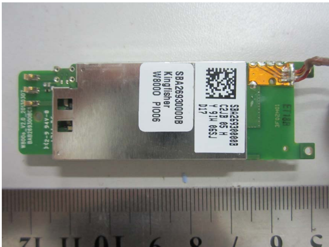
3. Mainboard rear view with shielding
