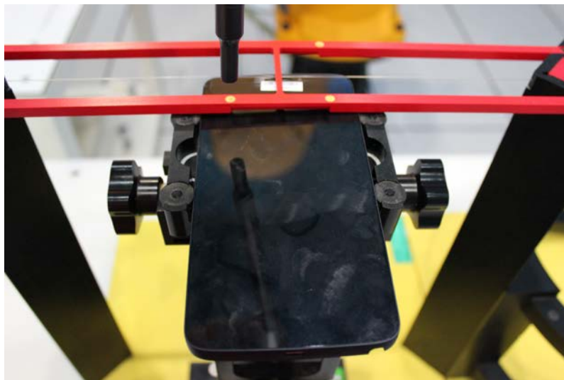
Picture 2: EUT Positioning for RF
