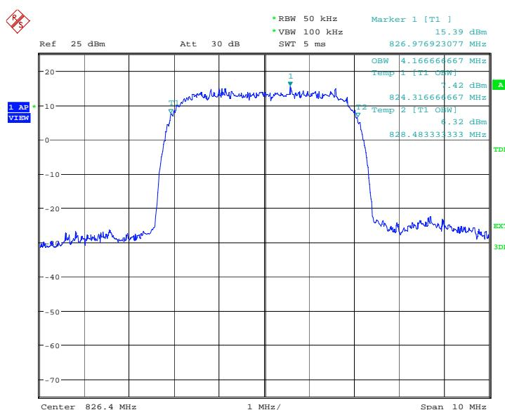
**Channel 4183-Occupied Bandwidth (99% BW)-QPSK**
