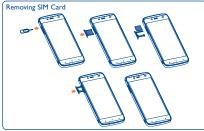
Before you install or remove the SIM card, use a pin to press the small cavity until the SIM cassette pops out.
