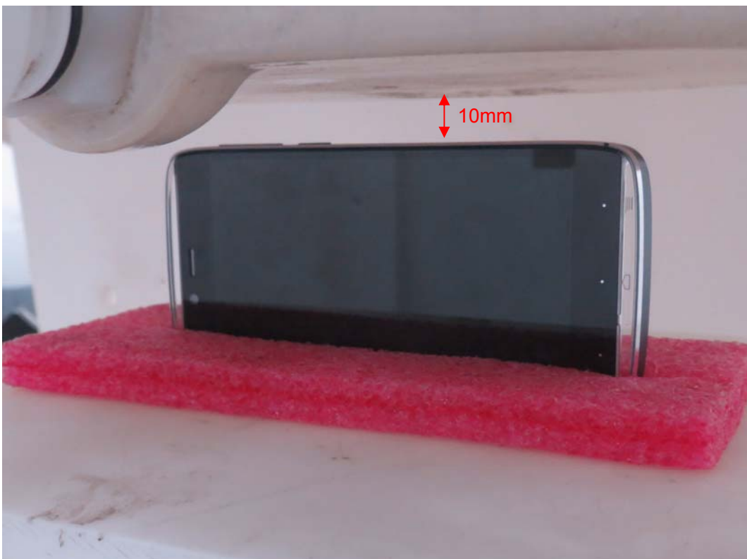
Picture 14: Right Edge, the distance from handset to the bottom of the Phantom is 10mm
