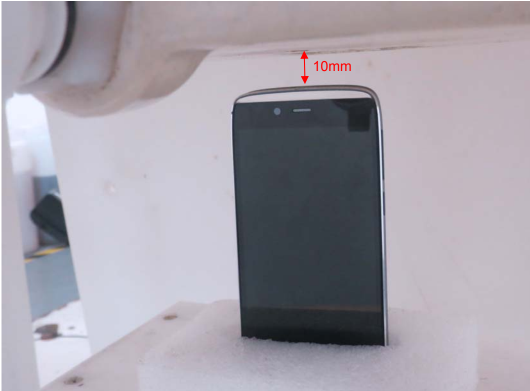
Picture 15: Top Edge, the distance from handset to the bottom of the Phantom is 10mm
