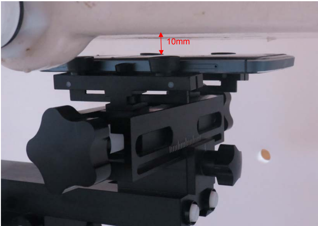
Picture 11: Back Side, the distance from handset to the bottom of the Phantom is 10mm
