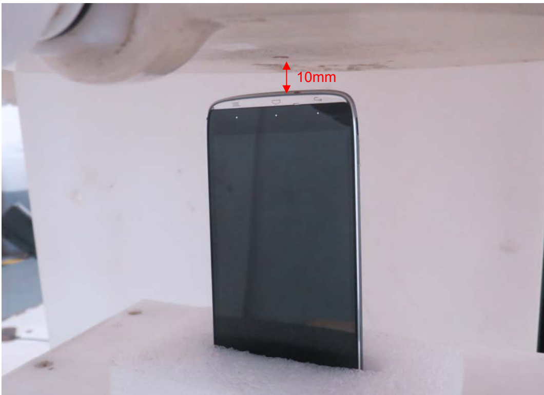
Picture 16: Bottom Edge, the distance from handset to the bottom of the Phantom is 10mm
