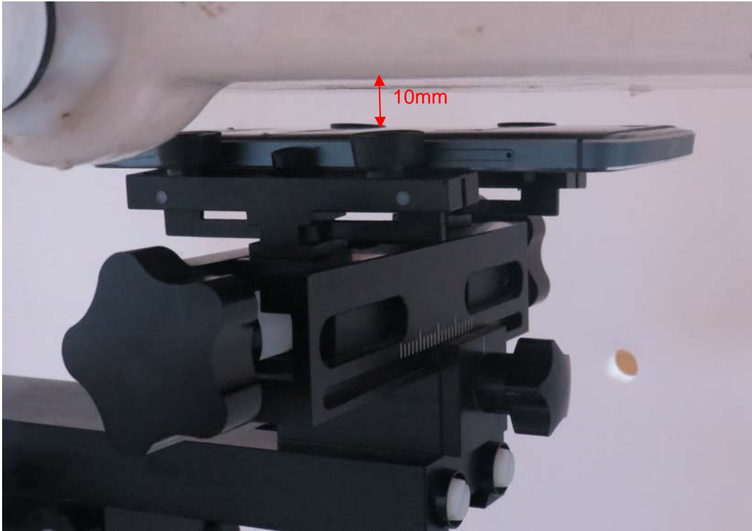
Picture 6: Back Side, the distance from handset to the bottom of the Phantom is 10mm
