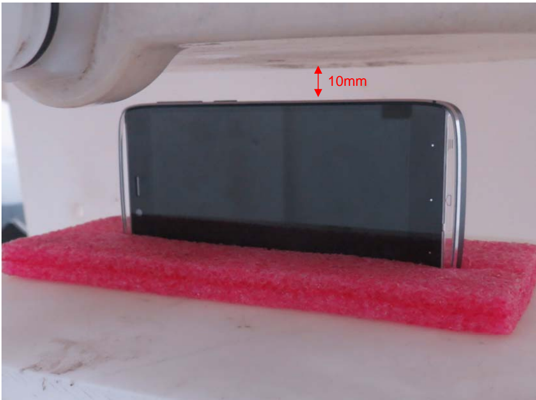
Picture 9: Right Edge, the distance from handset to the bottom of the Phantom is 10mm
