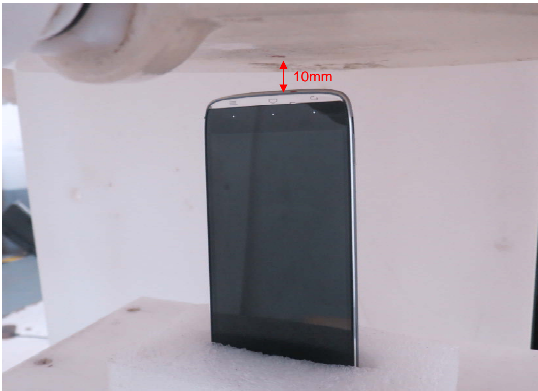
Picture 11: Bottom Edge, the distance from handset to the bottom of the Phantom is 10mm
