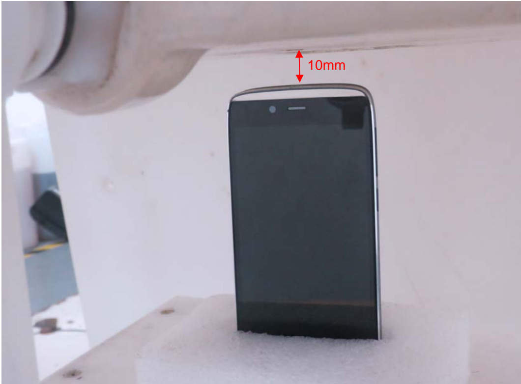
Picture 10: Top Edge, the distance from handset to the bottom of the Phantom is 10mm
