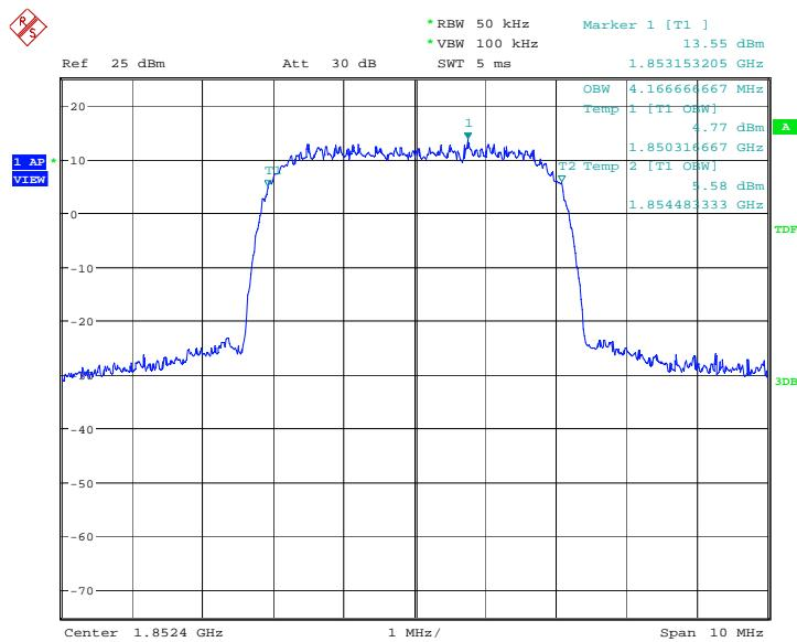
**Channel 9400-Occupied Bandwidth (99% BW)-16QAM-Antenna1**
