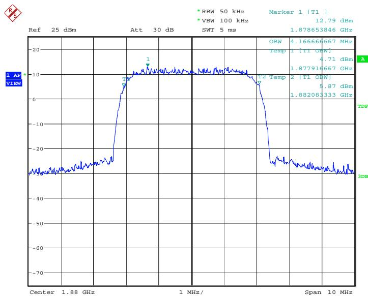
**Channel 9538-Occupied Bandwidth (99% BW)-16QAM-Antenna1**
