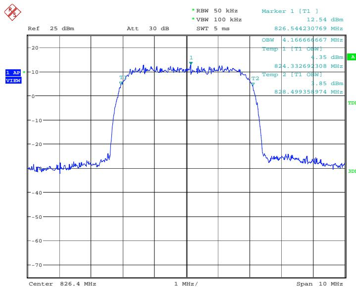
**Channel 4183-Occupied Bandwidth (99% BW)-16QAM-Antenna1**
