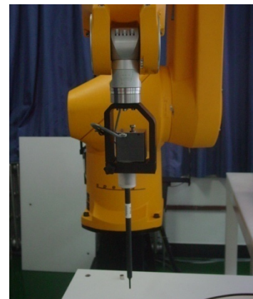
Picture C.3 E-field Probe
