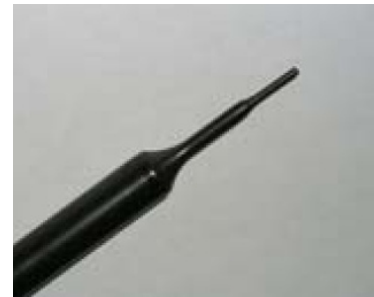
Picture C.2 Near-field Probe
