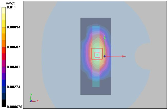
Figure 23 Body, Right Edge, GSM 850 GPRS (4Txslots) Channel 190
