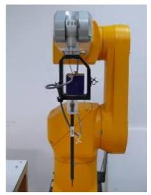
Figure 3. EX3DV4 E-field probe
