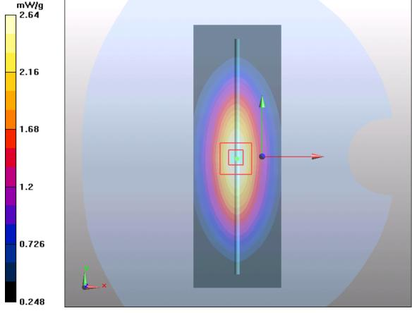
Figure 7 System Performance Check 835MHz 250mW
