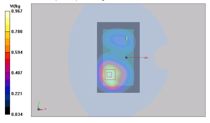
Figure 45 Body, Back Side, GSM 1900 EGPRS (4Txslots) Channel 810
