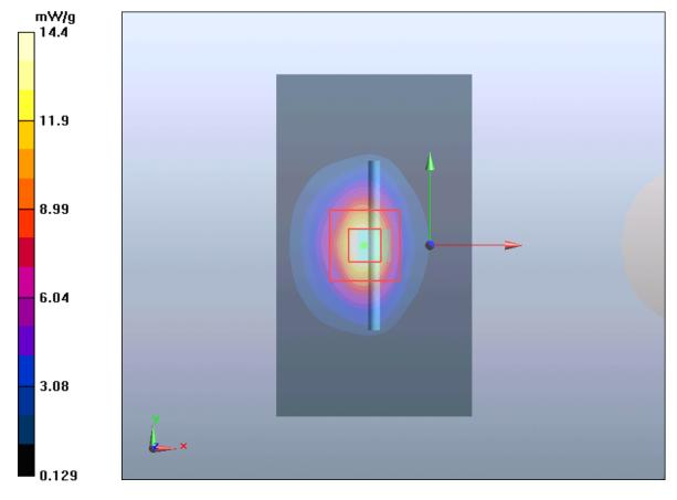
Figure 14 System Performance Check 2450MHz 250mW
