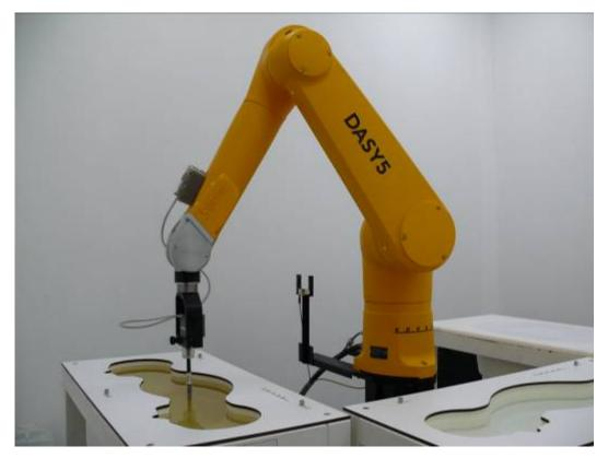
Picture 1: Specific Absorption Rate Test Layout
