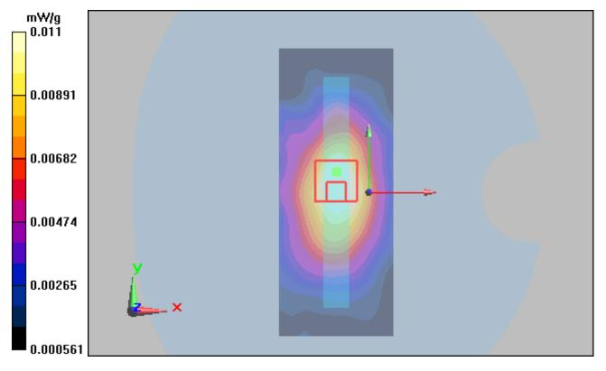
Figure 22 Body, Left Edge, GSM 850 GPRS (4Txslots) Channel 190
