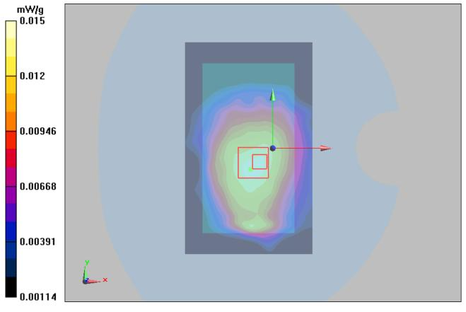
Figure 21 Body, Front Side, GSM 850 GPRS (4Txslots) Channel 190
