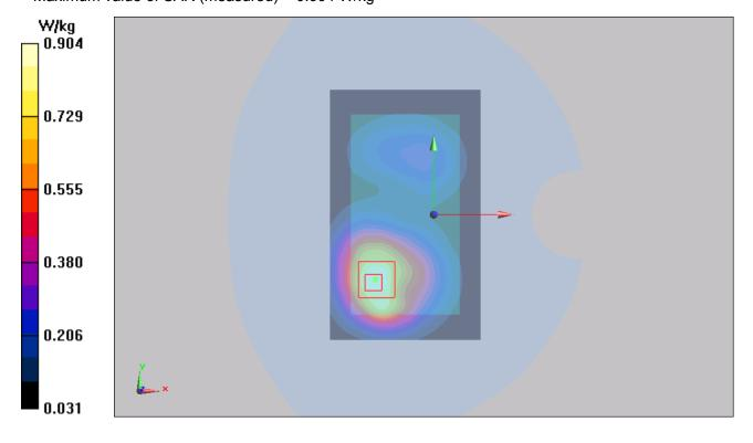
Figure 37 Body, Back Side, GSM 1900 GPRS (4Txslots) Channel 661
