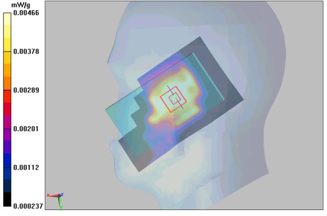
Figure 18 Right Hand Tilt 15° GSM 850 Channel 190
