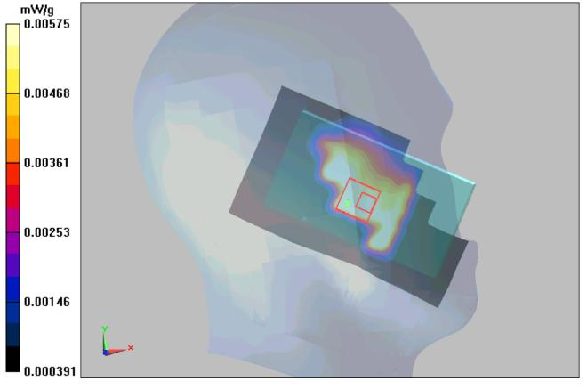
Figure 16 Left Hand Tilt 15° GSM 850 Channel 190
