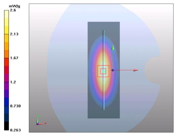
Figure 8 System Performance Check 835MHz 250mW
