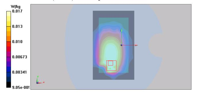
Figure 26 Body, Back Side, GSM 850 GPRS (4Txslots) Channel 190
