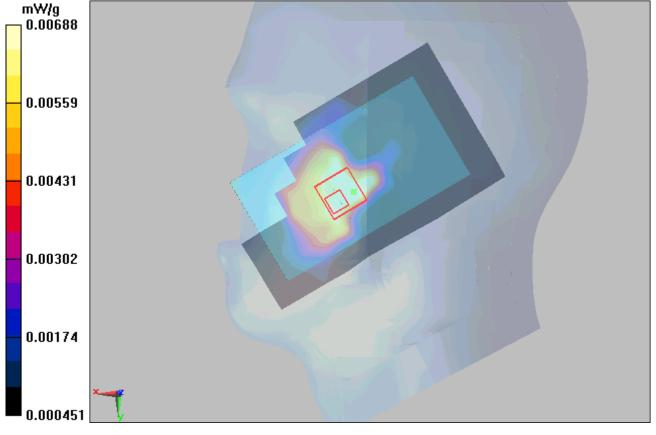
Figure 17 Right Hand Touch Cheek GSM 850 Channel 190
