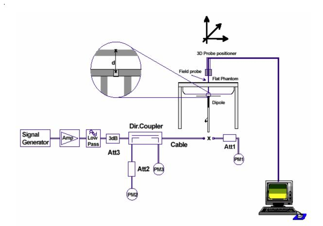
Figure 6 System Check Set-up
