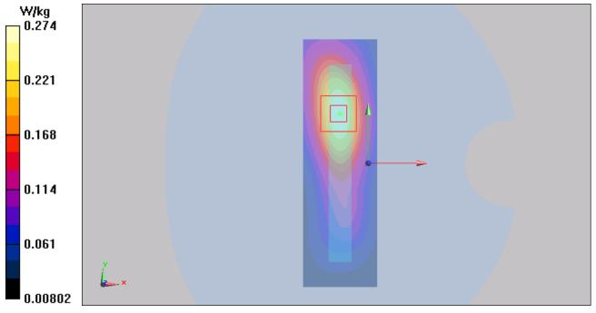
Figure 43 Body, Right Edge, GSM 1900 GPRS (4Txslots) Channel 661
