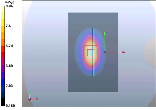
Figure 9 System Performance Check 1750MHz 250mW
