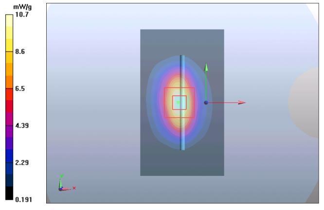
Figure 11 System Performance Check 1900MHz 250mW
