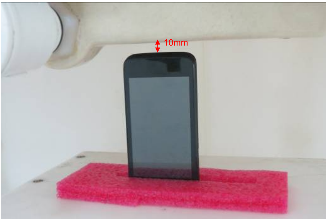
Picture 22: Bottom Edge, the distance from handset to the bottom of the Phantom is 10mm
