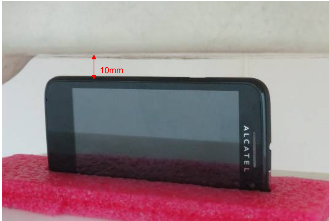
Picture 19: Left Edge, the distance from handset to the bottom of the Phantom is 10mm
