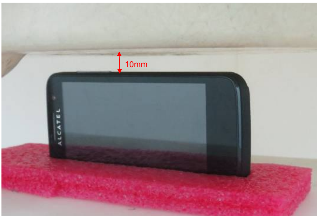
Picture 20: Right Edge, the distance from handset to the bottom of the Phantom is 10mm
