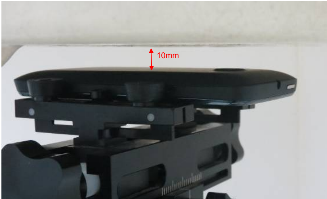
Picture 17: Back Side, the distance from handset to the bottom of the Phantom is 10mm
