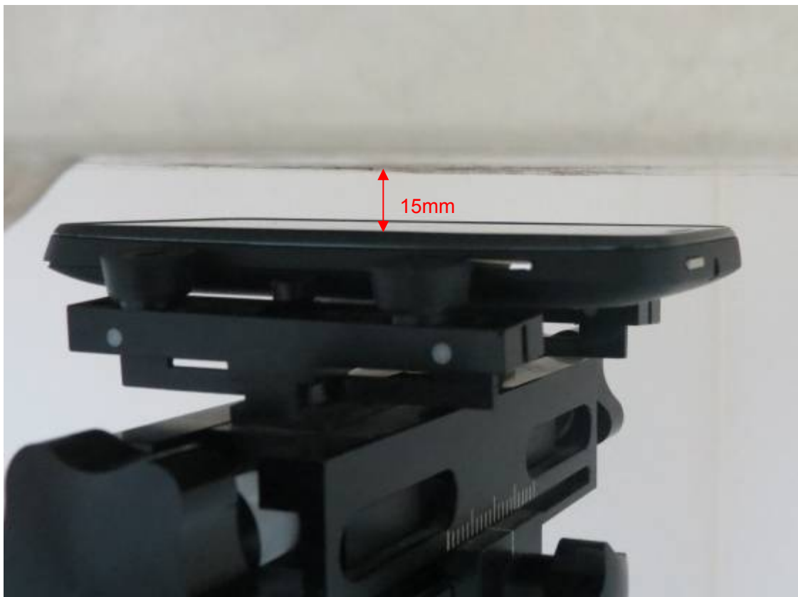
Picture 16: Front Side, the distance from handset to the bottom of the Phantom is 15mm
