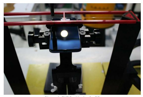
**Picture 2: EUT Positioning for RF**
