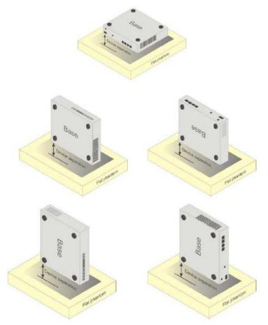
Picture D.5 Test positions for desktop devices
