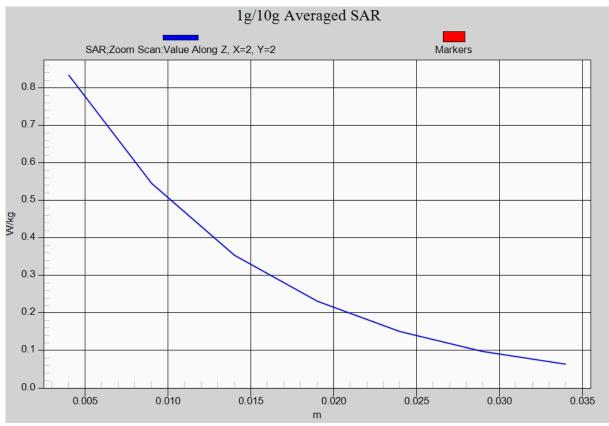
Fig. 7-1 Z-Scan at power reference point (WCDMA1900 CH9400)
