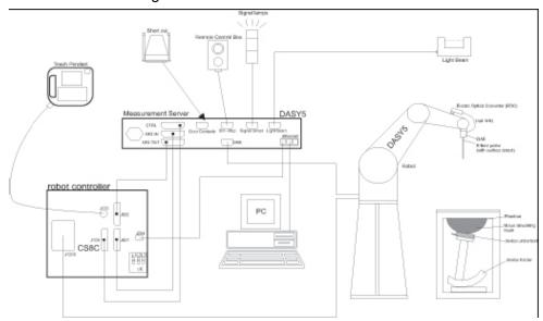
Picture C.1 SAR Lab Test Measurement Set-up
