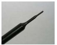
Picture C.2 Near-field Probe
