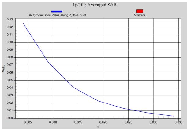
Fig. 10-1 Z-Scan at power reference point (2450 MHz CH1)
