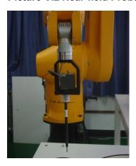
Picture C.3 E-field Probe
