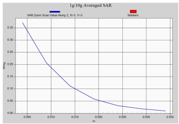
Fig. 9-1 Z-Scan at power reference point (2450 MHz CH1)
