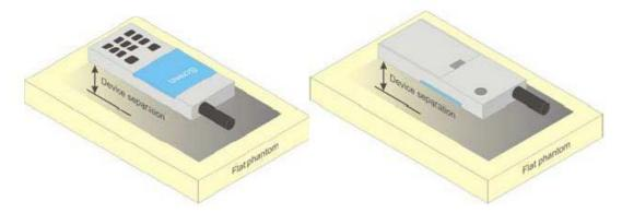
Picture D.4 Test positions for body-worn devices
