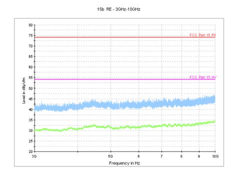
Figure A.6 Radiated Emission from 3GHz to 4GHz (Set.2, Charging mode)
