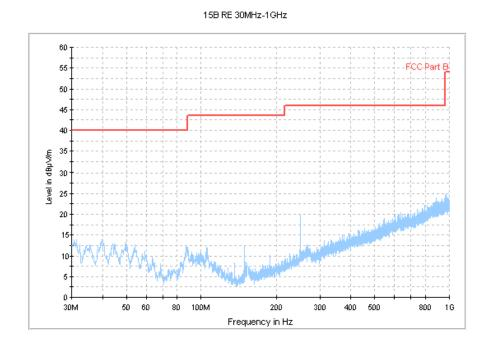
Figure A.4 Radiated Emission from 30MHz to 1GHz (Set.2, Charging mode)
