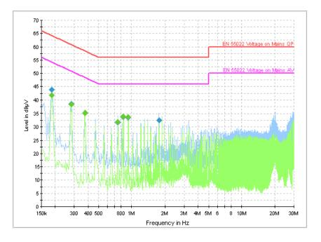
Figure A.10 Conducted Emission (Set.1, USB mode)
