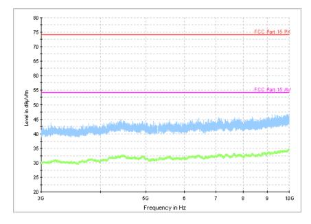
Figure A.9 Radiated Emission from 3GHz to 4GHz (Set.3, Charging mode)
