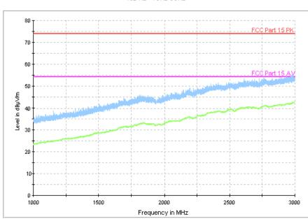
Figure A.8 Radiated Emission from 1GHz to 3GHz (Set.3, Charging mode)
