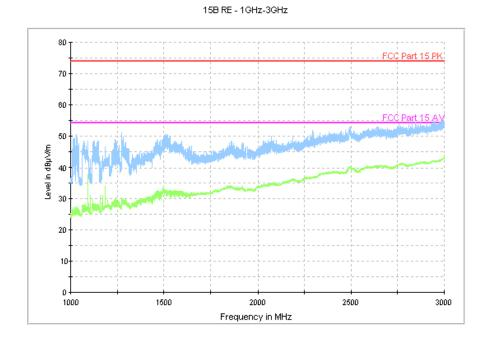
Figure A.2 Radiated Emission from 1GHz to 3GHz (Set.1, USB mode)
