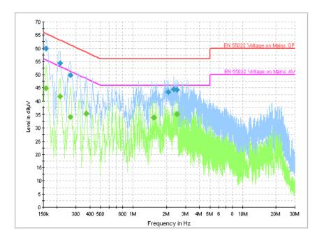
Figure A.12 Conducted Emission (Set.3, Charging mode)
