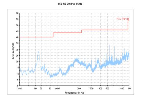
Figure A.1 Radiated Emission from 30MHz to 1GHz (Set.1, USB mode)
