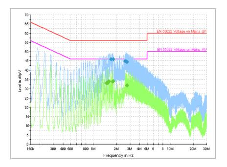
Figure A.11 Conducted Emission (Set.2, Charging mode)
