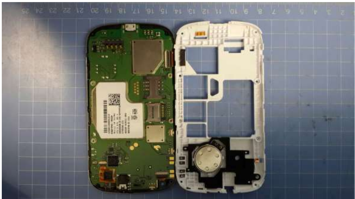
Mobile Phone Disassembly
