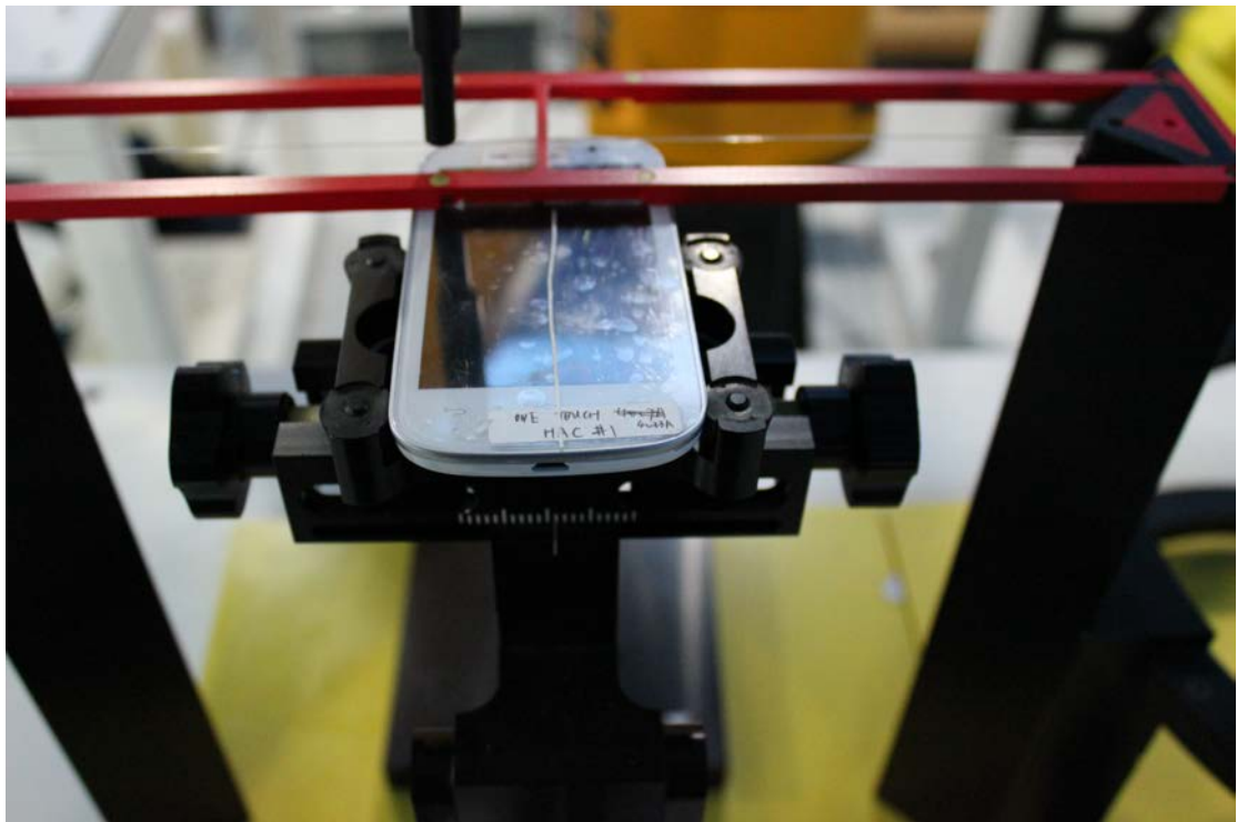
Picture 2: EUT Positioning for RF
