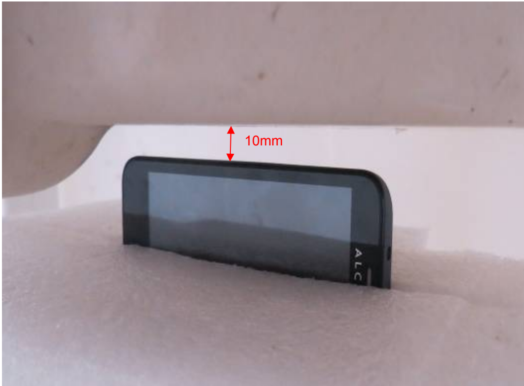
Picture 19: Left Edge, the distance from handset to the bottom of the Phantom is 10mm
