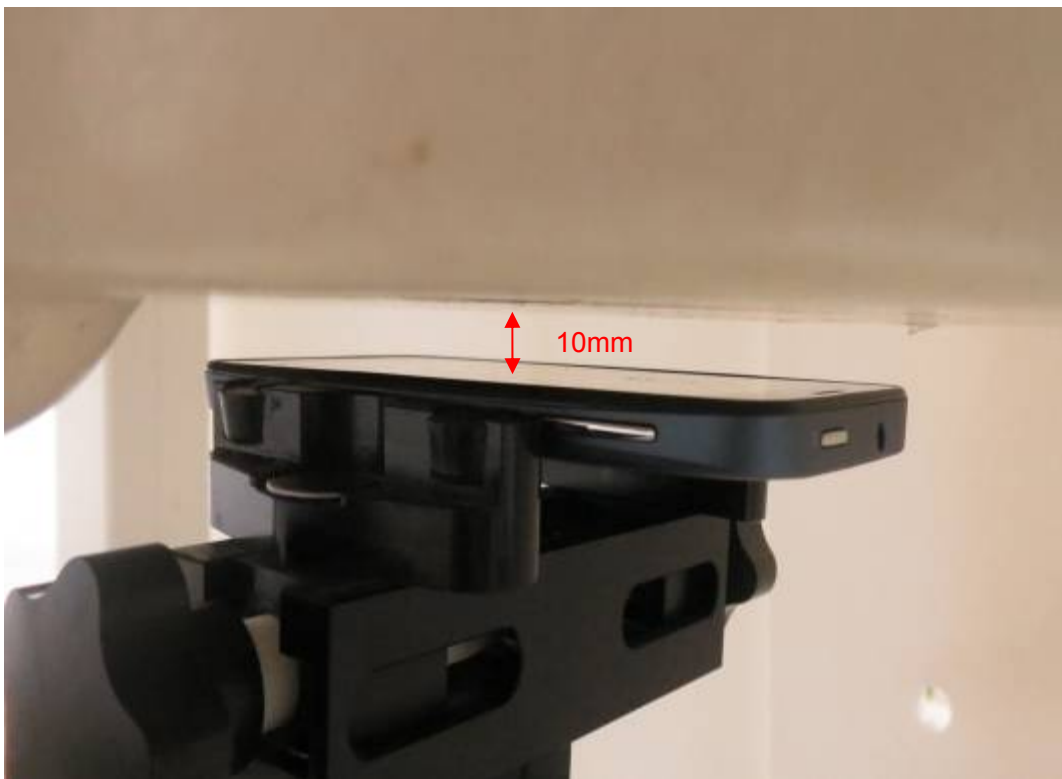
Picture 18: Front Side, the distance from handset to the bottom of the Phantom is 10mm
