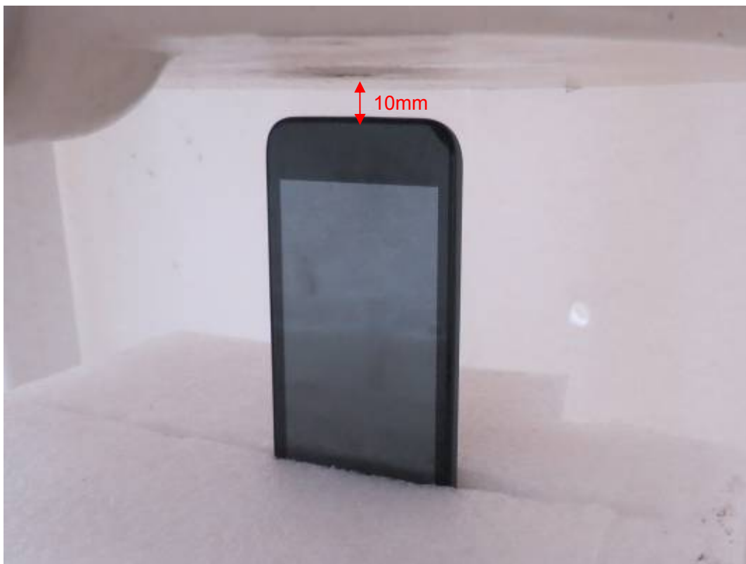
Picture 22: Bottom Edge, the distance from handset to the bottom of the Phantom is 10mm
