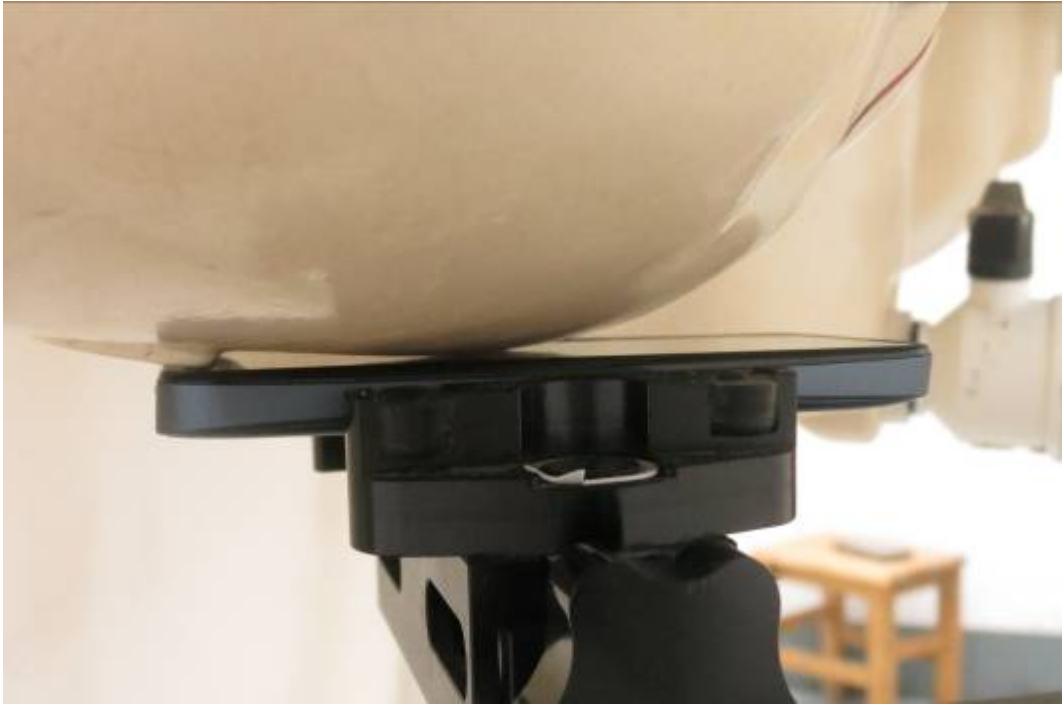
Picture 13: Right Hand Touch Cheek Position
