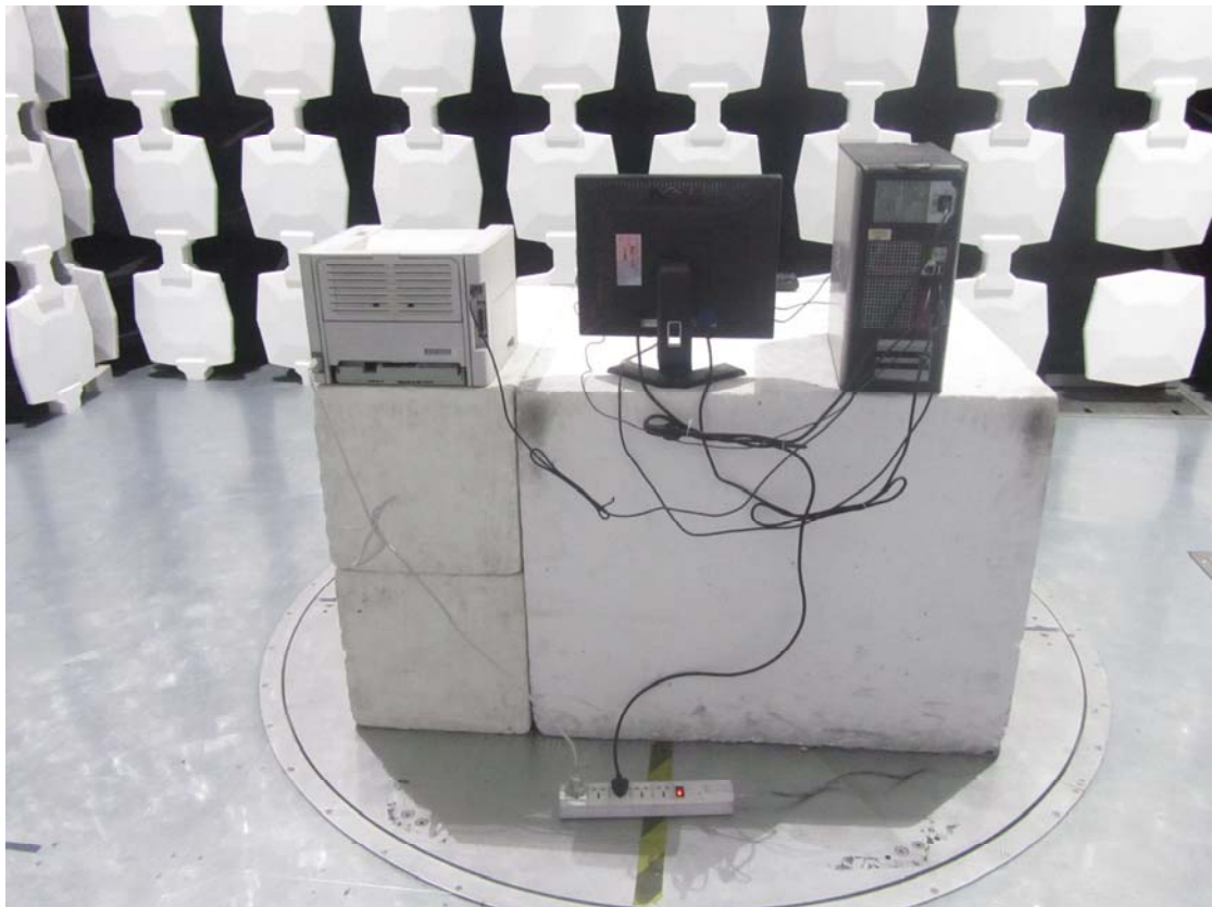
Radiated Spurious Emission
