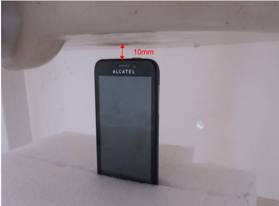
Picture 21: Top Edge, the distance from handset to the bottom of the Phantom is 10mm
