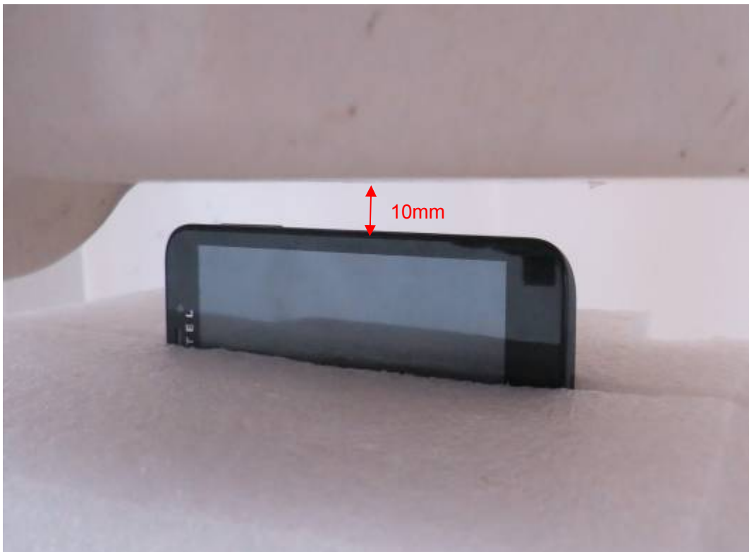
Picture 20: Right Edge, the distance from handset to the bottom of the Phantom is 10mm
