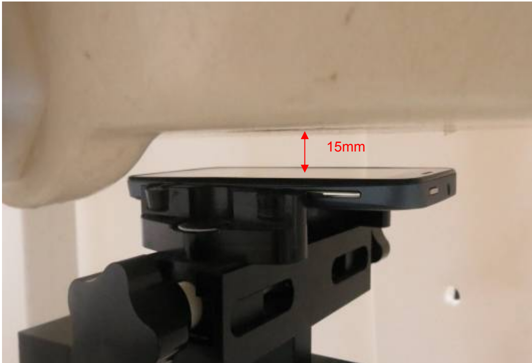
Picture 17: Front Side, the distance from handset to the bottom of the Phantom is 15mm
