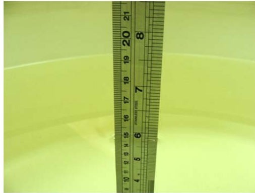
Fig 6.1 Photo of Liquid Height for Body SAR
