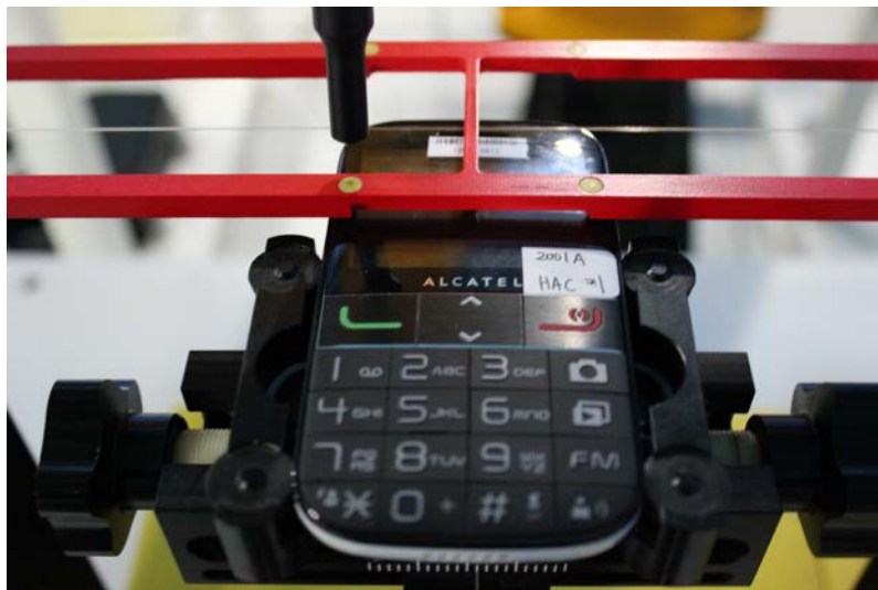
Picture 2: EUT Positioning for RF
