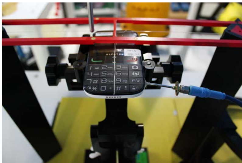
Picture 3: EUT Positioning for T-coil
