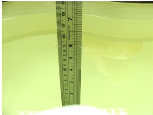
Fig 6.1 Photo of Liquid Height for Head SAR
